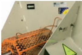
External grease fittings to aid maintenance
