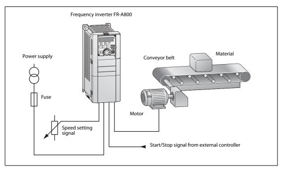
The configuration is as follows: The belt is started and stopped by an external controller (for example a PLC). The speed of the motor and thus of the conveyor belt can be adjusted with a setpoint potentiometer.
