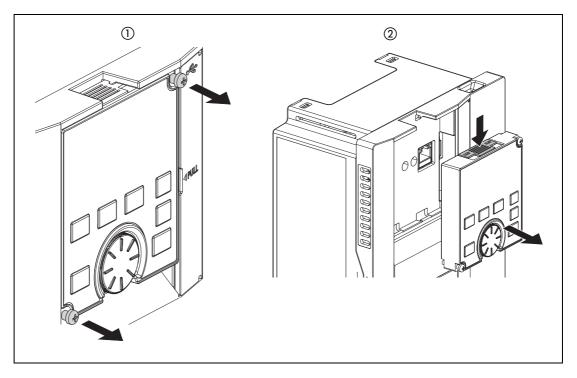
To reinstall the parameter unit, align its connector on the back with the PU connector of the inverter, and insert the parameter unit. After confirming that the parameter unit is fit securely, tighten the screws. (Tightening torque: 0.40 to 0.45 Nm)
