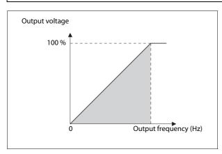
The speed of the connected motor can be adjusted continuously by changing the output voltage and frequency of the inverter.
