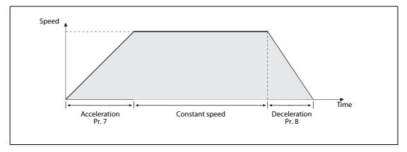
In this example we are going to use an FR-A800 series inverter to power and control the belt using the speed/time pattern shown in the graph above.
