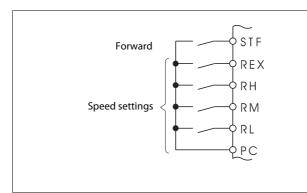
Example for connection of the inverter's RH, RM, RL and REX terminals (in source logic).
