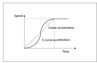
If the material on the belt still shifts when stopping and starting even with a gentle acceleration curve you can solve the problem by programming an S-curve for acceleration and deceleration, as shown in the graph on the left.
