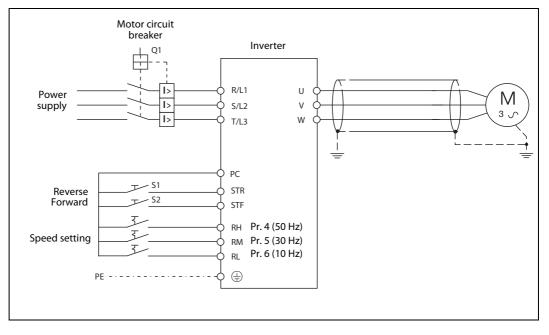
Some external components like pushbuttons and switches are required for this method but it has advantages over performing the test with the parameter unit:
