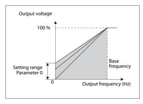
You can use parameter 0 to achieve better performance for starting the motor under load. The base frequency is set in parameter 3.
