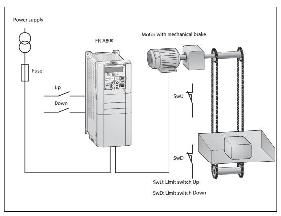
In the wiring diagram on the next page the mechanical brake is controlled via the RUN terminal. The frequency at which the brake is released can be set with parameter 13.
