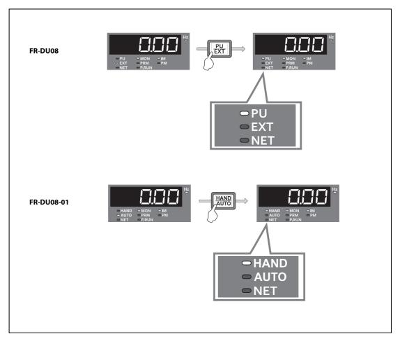
Pressing PU/EXT when the inverter is in PU operation mode switches the system to external operation mode and the EXT indicator lights up.
