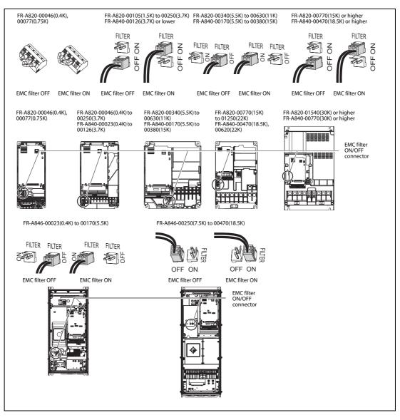
The connector must always be installed, either in the ON position or in the OFF position.
