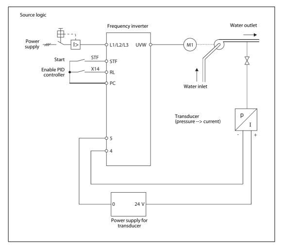
In addition to the basic parameters you must also set the following parameters for this configuration:
