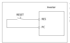
This example shows how to wire the RES terminal for positive logic.
