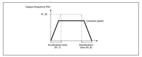
Parameter 7 sets the acceleration time for the drive. The value defines the time in seconds in which the drive will be accelerated up from 0 Hz to the frequency preset in parameter 20.
