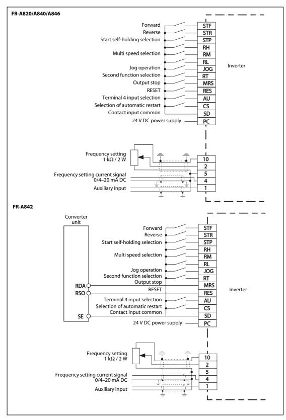
The following illustration shows the connection of the control terminals when sink logic (factory default for FM types) is used. The inputs are connected to 24 V DC.
